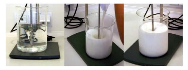
**Figure 1. a:** Propeller stirrer properly positioned in mixing vessel. **b:** Addition of Aquarius<sup>™</sup> film coating system powder to the solvent solution. **c:** Mixing for 60 minutes.
