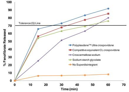
Figure 1. Dissolution profile of fenofibrate tablets (at initial time) in 0.025M SLS medium
