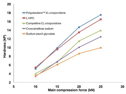
Figure 1. Effect of compression force on hardness of acetaminophen ODTs
