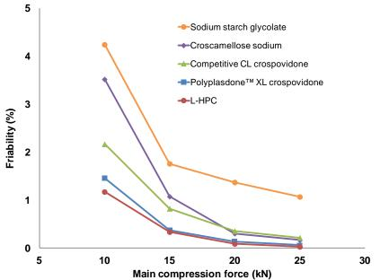
Figure 2. Effect of compression force on friability of acetaminophen ODTs
