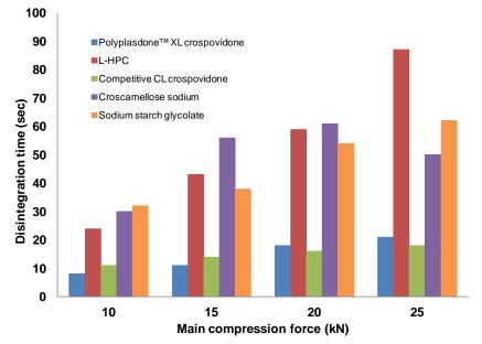
Figure 3. Effect of compression force on disintegration time of acetaminophen ODTs
