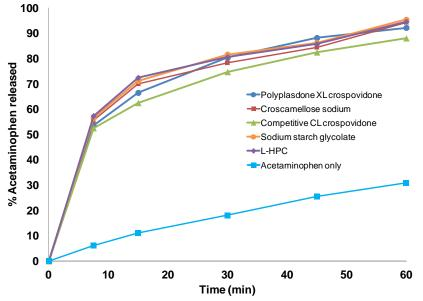
Figure 4. Dissolution profile of acetaminophen ODT in pH 5.8 phosphate buffer
